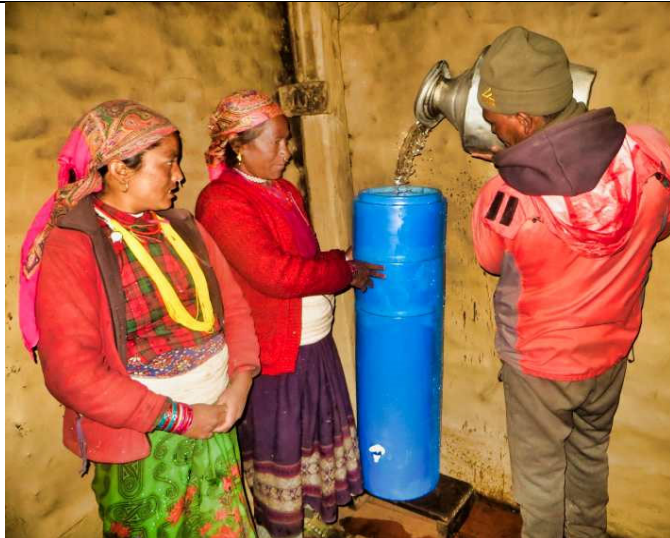
PIC.134. Karna is helping and teaching two Pere women how to fill water regularly in the SSWF to keep the sand constant wet for best and clean drinking water quality.
